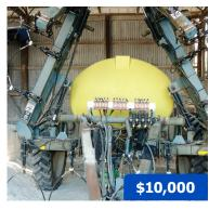
2010 Dalton Ag DLQHD35, 15 row side dress rig with 1200 gal. poly tank, 37.5 ft booms, 30 in. nozzle spacing, 3-sections, Y-drops, JD rate controller for 2630 screen. Raven rate controller and display still available. Coulters and shanks available for injecting nitrogen.
