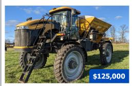
**2014 AGCO RG1300 RoGator**, 1892 hours, AGCO 8.4L 330 hp turbo diesel engine, 4WS, painted 409 SS New Leader L4000G4, Raven Viper Pro, Phoenix 300 GPS, parallel swathing, air ride seat, A/C, beacon lights, fenders, electric roll tarp, Michelin 380/90R46 tires (front 45%, rear 35% remains).
