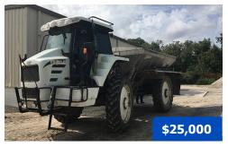
**2010 GVM 9275 Prowler,** 5000 hours, Cummins QSB6.7L 275 hp diesel engine, Funk DF250 10-speed powershift trans., 304 SS New Leader L3220G4 8 ton spreader, AgLeader Insight, A/C, AM/FM radio, air ride seat, Firestone floater tires (50% remains). New exhaust pipe and BOC installed, 2020.
