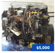
2010 4660 SpraCoupe Perkins Diesel Engine 1104D, 874 hours, 4 cylinder, 4.4L (269 in.³), 125 hp (93 kW) at 2200 rpm. Engine includes: alternator, starter injection pump, turbo charger, and primary fuel filter and housing. (PA)
