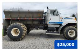
**1996 International Spreader,** DT466 turbo diesel engine, Roadranger manual 10-speed trans., 304 SS New Leader L2020GT-12 spreader, brand new InCommand 800 with 6500 GPS receiver, front 48/25.00 tires (40% remains), rear 66/43.00/25 right (50% remains) left (30% remains).
